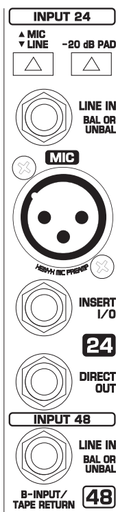
Fig. 7.8: A and B-channel input section
