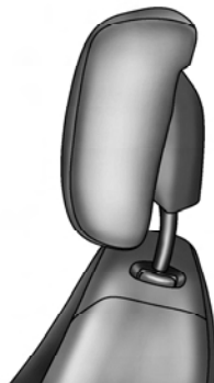
Active Head Restraint (Normal Position)
