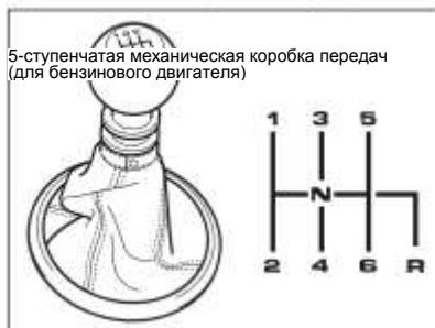
6-speed manual transaxle (for Diesel engine) 80J2033
