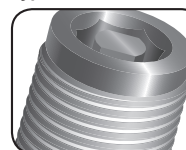
Fine thread (example: steel 290 g/40 L CO 2 cylinders and steel 450 g/60 L CO 2 cylinders)
