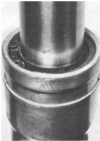
7.2a Remove seal retaining circlip
