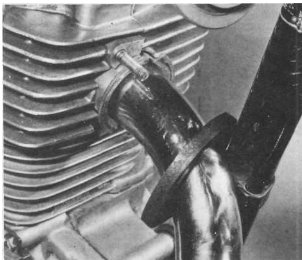
40.4c ... then fit exhaust system. Note packing pieces
