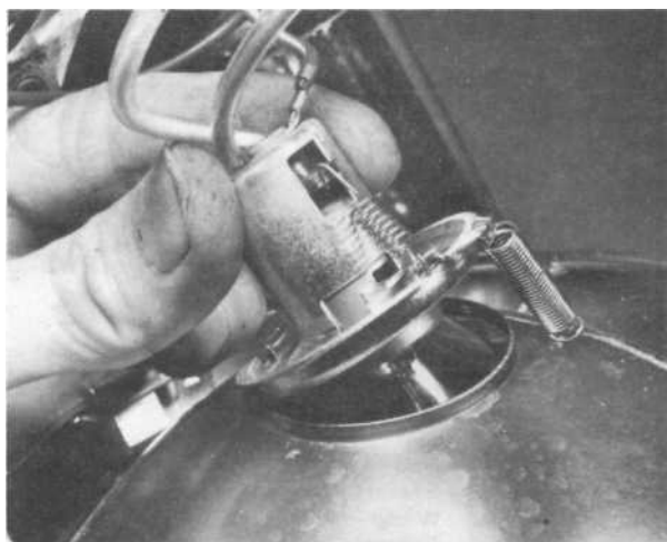
6.2 Bulb is mounted in spring-loaded holder - early models
