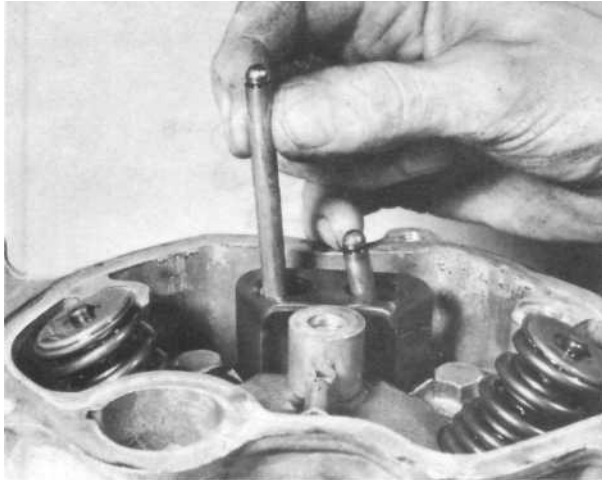
7.2c Withdraw the pushrods, noting which is inlet and exhaust
