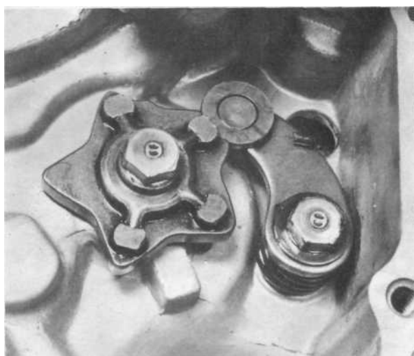
35.2c Fit camplate and tighten bolt
