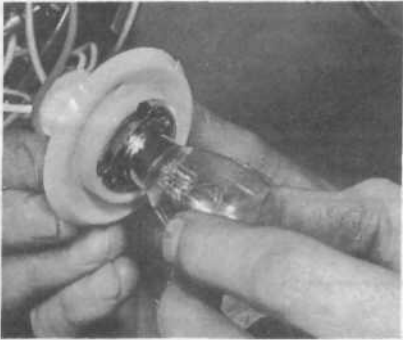
1.7e ... ensure bulb locating tangs engage with matching slots in holder
