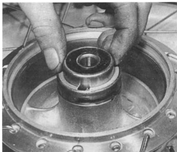
6.3b Bearing sealed surface must face outwards
