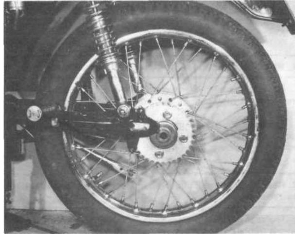
9.3c Wheel can be removed from frame
