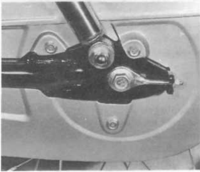
1.7a Chain enclosure is secured by three bolts at the rear on BR-E/F and BR-J models ...
