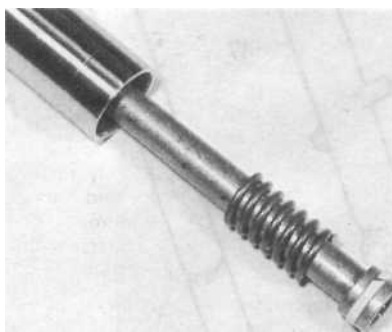
21.2b ... and insert damper assembly into top of stanchion
