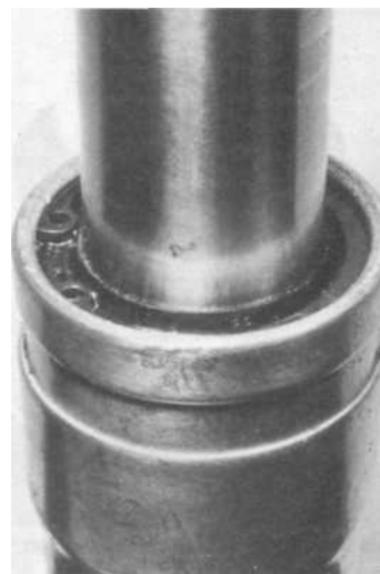
7.6e Renew seal and replace the circlip
