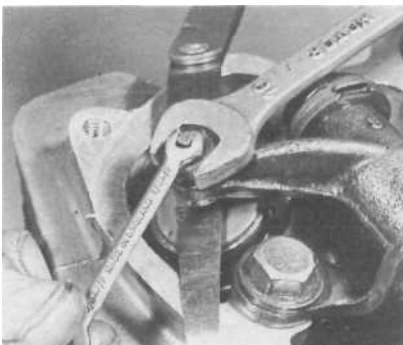
Set clearance so that the feeler gauge is a sliding fit
