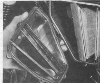
4.2 Air filter cover is retained by six screws - note sealing gasket
