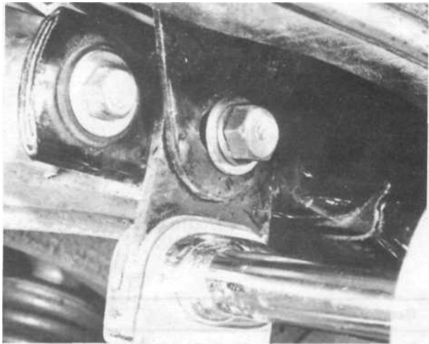
5.3 Seat is retained by two bolts at rear
