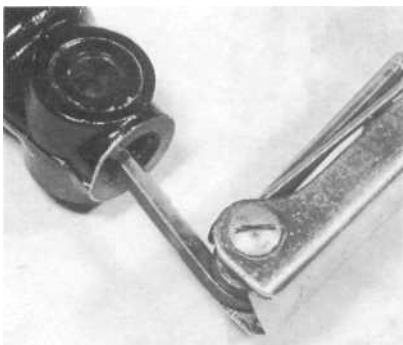
20.2 Unscrew damper rod Allen screw to release stanchion from lower leg
