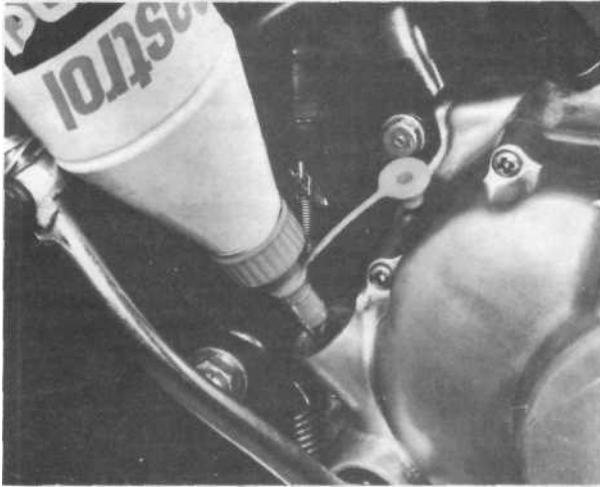
40.6 Refill crankcase to correct level with engine oil
