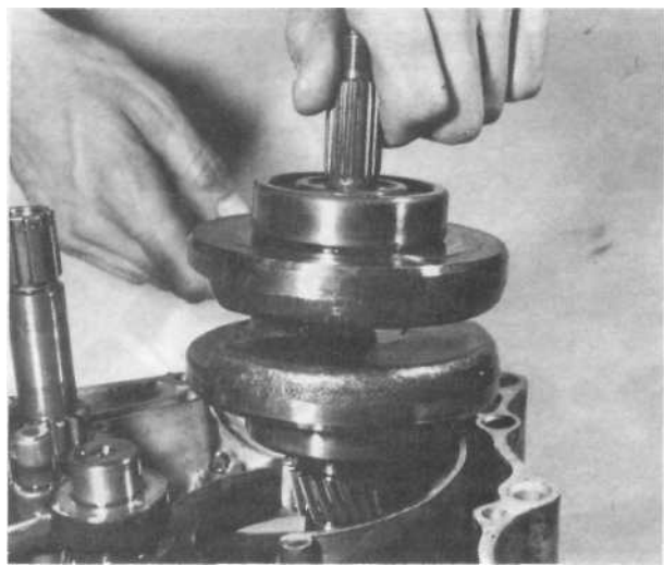
16.1b Crankshaft assembly lifts easily out of case
