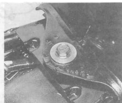
11.1 Petrol tank rear mounting is secured by a single bolt
