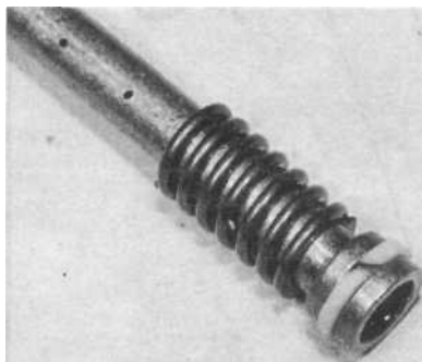
21.2a Fit rebound spring and piston ring to damper rod ...
