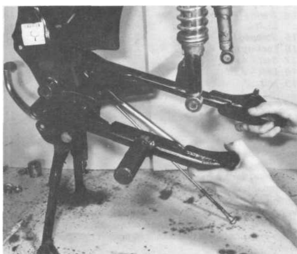
11.4c Remove swinging arm from frame
