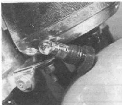
10.1 Instrument bulb holders are a push-fit in base
