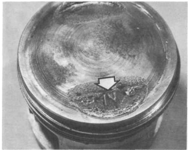
39.2 Cutout for inlet valve is marked appropriately
