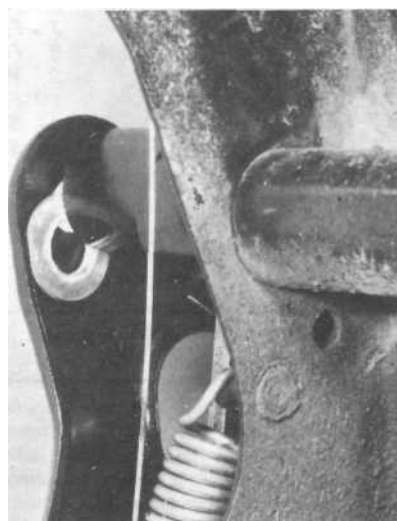
1 1.4d ... noting washers each side of exhaust mounting bracket
