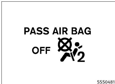
Front passenger air bag status light
