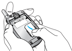
To insert the SIM card
