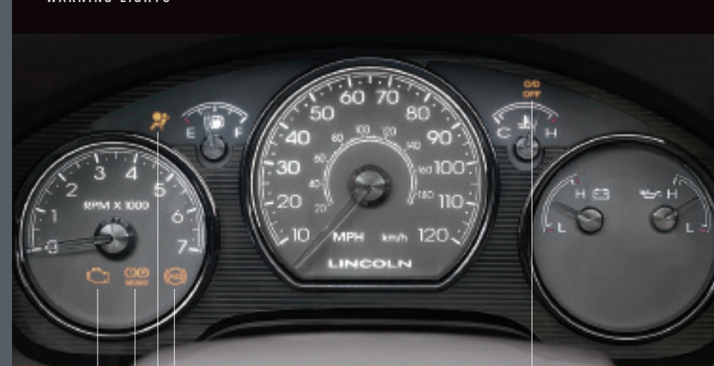
1. SERVICE ENGINE SOON LIGHT 2. BRAKE SYSTEM WARNING 3. AIRBAG READINESS 4. ABS WARNING LAMP 5. OVERDRIVE OFF
