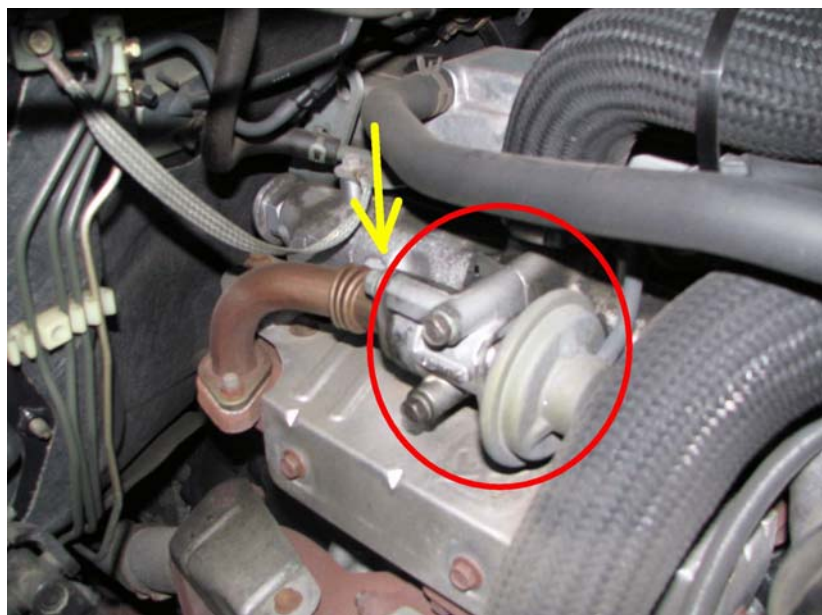
Figure 35: Location of EGR valve on Delica (circled). If the valve has to be blanked off, do so by inserting a plate at the arrow point.
