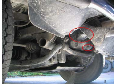
Figure 25: Oil filter (top left) and drain plug (bottom right).
