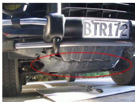
Figure 24: Remove this steel guard.
