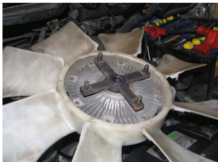
Figure 31: Fan and thermal clutch after removal.
