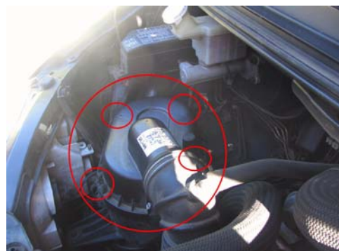
Figure 27: Housing for Air filter. Release the four clamps circled.
