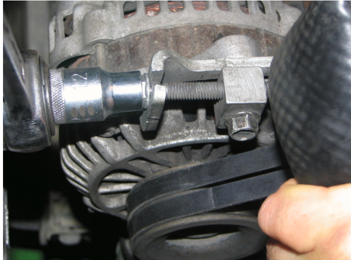
Figure 30: Tension the alternator belts by tightening (clockwise) this screw. Make sure that the second screw (right) is slack at this time. When the belts are tight enough, then tighten this second screw to lock the mechanism in place.
