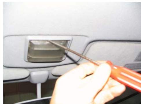
Figure 34: Replace an interior light by lifting off the cover at the long edge.
