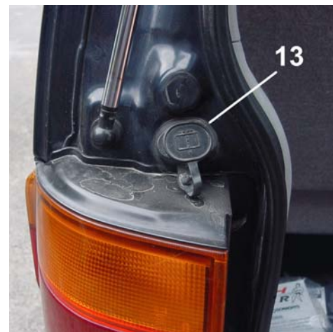
Figure 6: Fill location for rear windscreen water spray.
