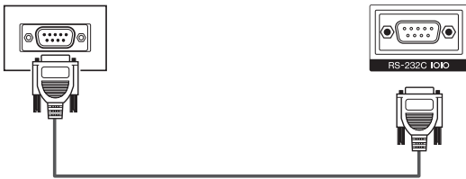
RS-232C serial control cable (cross type)
