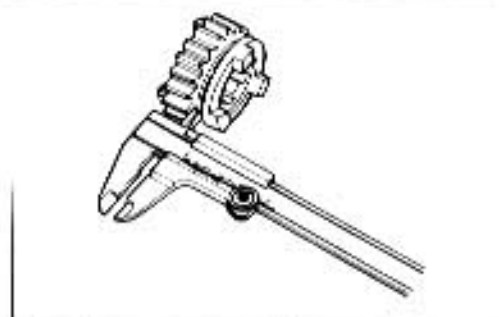
Checking groove width
