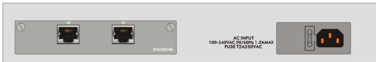
Figure 3-2 ES-4024 Rear Panel: AC model
