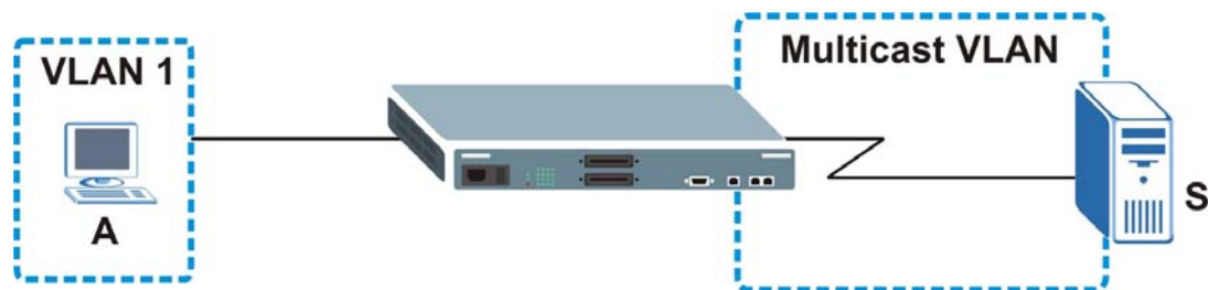
Figure 99 MVR Multicast Television Example
