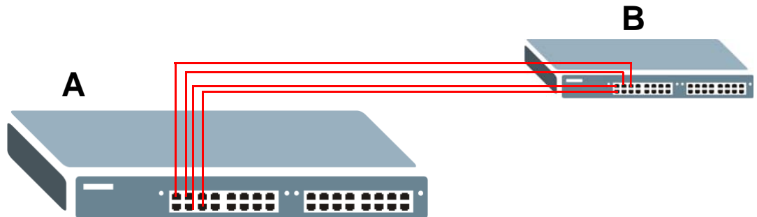
Figure 85 Trunking Example - Physical Connections
