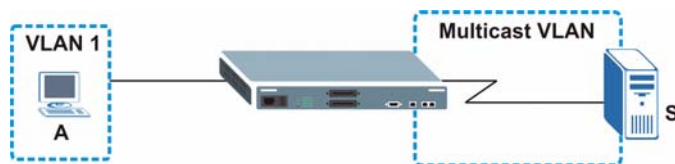
Figure 82 MVR Multicast Television Example
