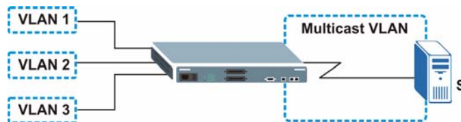
Figure 81 MVR Network Example
