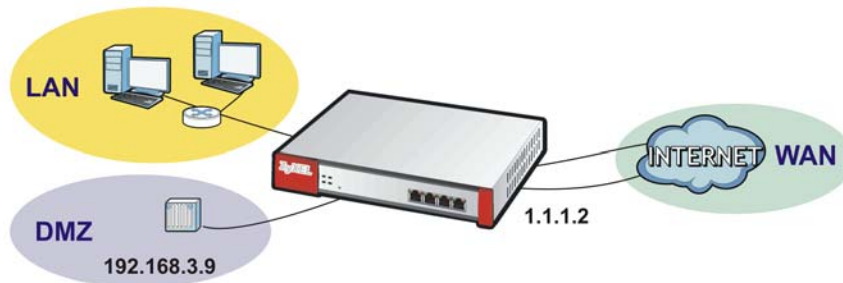
Figure 48 IPPBX Example Network Topology
