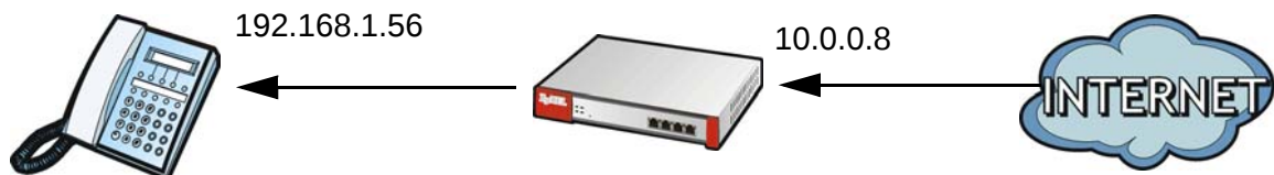
Figure 46 WAN to LAN H.323 Peer-to-peer Calls Example
