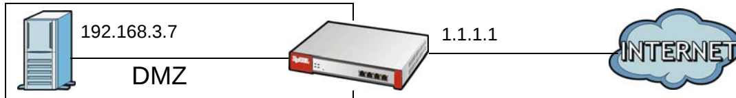
Figure 45 Public Server Example Network Topology
